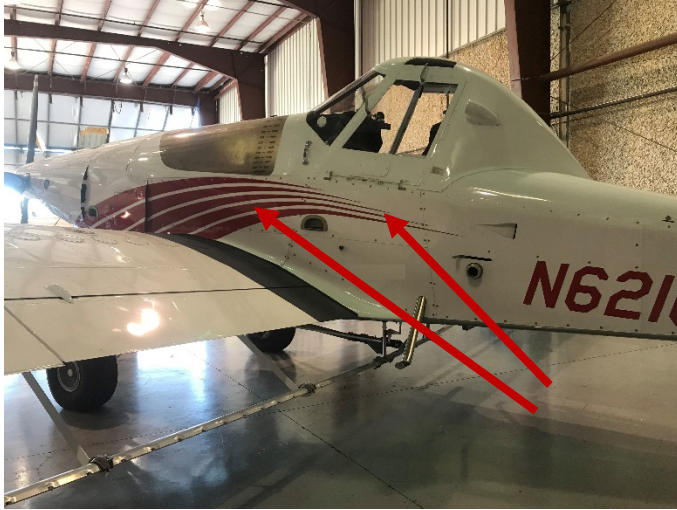
Figure 72-1 Emergency Fuel Pump Location
